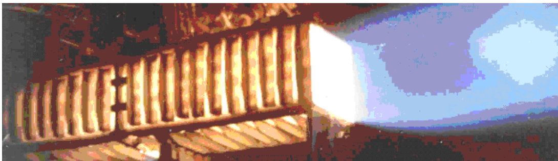
Figure 13: Massive Niobium scramjet combustor under Mach 6 flight conditions testing (MAI).
